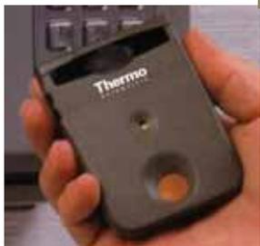
The EPD<sup>®</sup> Mk2 is suitable for use as a single stand-alone dosimeter or as part of a comprehensive dosimetry management system using renowned hardware and software packages. The high quality and standard battery contribute to competitive lifetime costs.
